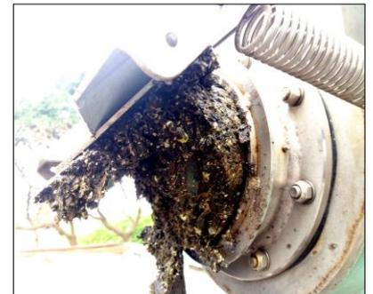
The solids removal efficiency of the separator can reach 80 % depending on the nature of the wastewater and since it is able to remove organic suspended matter, it can remove up to 20 % - 50 % of the BOD<sub>5</sub> load, depending on the wastewater type. The **MBF** can also be used after a coagulation & flocculation stage as a very **effective ‘physical-chemical’ separation process** that can provide COD removal in excess of 50% in certain applications.
