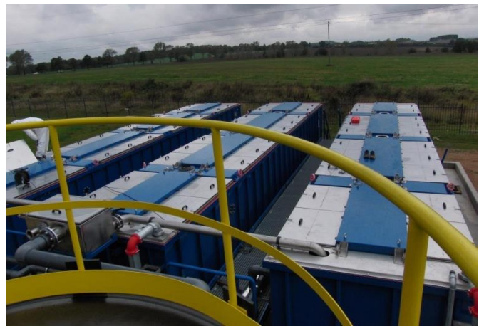
Multiple Packaged Bio Plants operating in Parallel in the Wastewater Treatment Plant of the "Colgate-Palmolive" Factory
